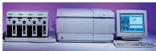
Figure 3. Hardware for the Affymetrix platform. The fluidics station (on the left), for washing and staining, can process up to 4 *GeneChips* simultaneously in about 90 minutes. The epifluorescence scanner (middle) has a resolution of 3 microns and scans each chip twice over 10 minutes. Both machines are software-controlled.
